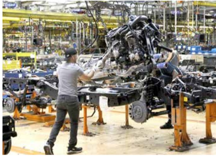
Workers put engines on the frame at a Ford Truck Plant in Michigan (file photo)
