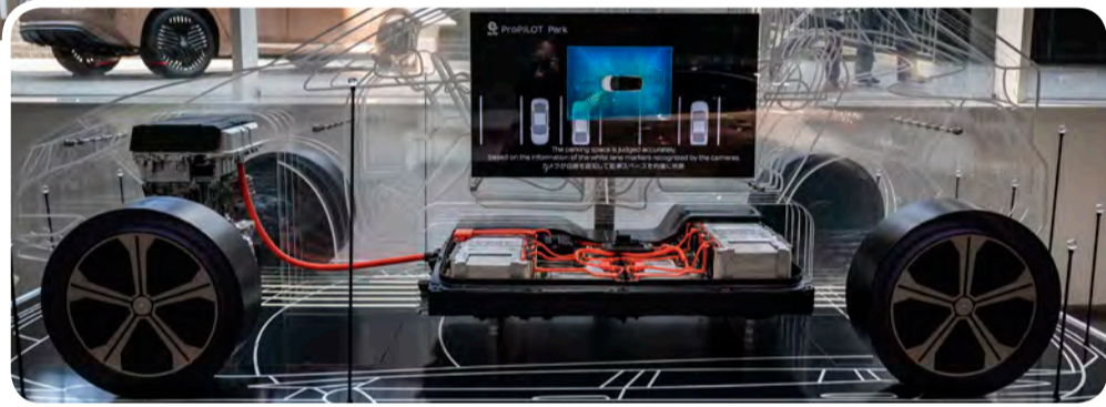
A cutaway display of the battery and engine system of one of Nissan's electric vehicles (EV) at the global headquarters of Japanese automaker Nissan Motor in Yokohama, Kanagawa prefecture.
