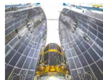
Hakuto-R Mission 1 lander stored in the fairing of SpaceX's Falcon 9 rocket
