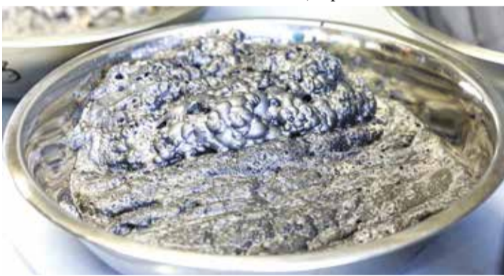
Recycled graphite attached to air bubbles and rising to the surface of the flotation cell at the graphite recycling system in a laboratory of the Helmholtz Institute Freiberg for Resource Technology in Freiberg, eastern Germany
