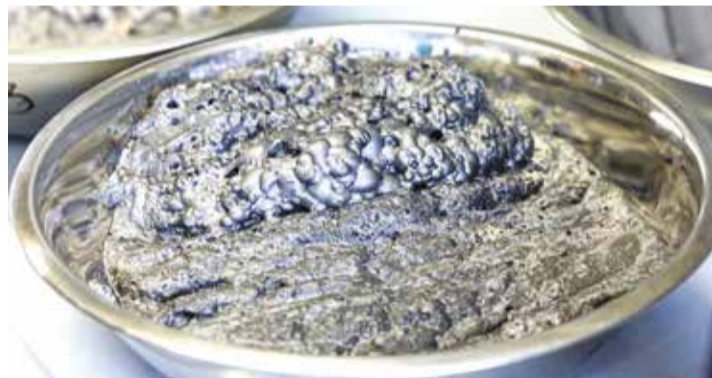
Recycled graphite attached to air bubbles and rising to the surface of the flotation cell at the graphite recycling system in a laboratory of the Helmholtz Institute Freiberg for Resource Technology in Freiberg, eastern Germany
